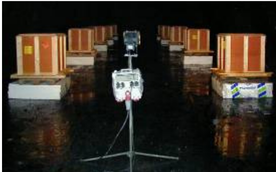
10-t TNT bare charge, distributed in 10 cubes of 1 ton each
