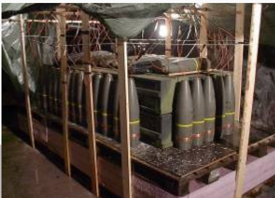
Mixed storage: propellants surrounded by 155 mm shells
